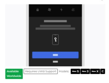
Ultrawide band (UWB) technology is now available for Phone Key. So your vehicle and Phone Key can communicate with greater accuracy to more responsively lock, unlock, and open Automatic Doors.
